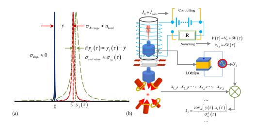
Figure 1 (color online). (a) Schematic diagrams of the noise of the AFS. (b) NSC experimental setup in an AFFS. In Fig.1 (b), the corresponding parameters are detected synchronously, then their FSCs are solved by the NSC method. An experiment is demonstrated on AFFSs by second-order Zeeman shift, where additional current noise of solenoid coil is introduced to affect the magnetic intensity of the AFFS, its FSC is evaluated from the sequences of  $\{y_j\}$  and  $\{\delta V_j\}$ .
