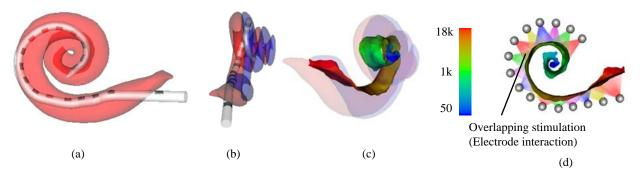
**Figure 1.** Panels (a) and (b) show a CI electrode array superimposed on the scala tympani (red) and scala vestibuli (blue) cavities of the cochlea in posterior-to-anterior and lateral-to-medial views, respectively. Panel (c) shows the scalae and neural activation region color-coded by place frequency in Hz. Panel (d) illustrates overlapping stimulation patterns (electrode interaction) from the implanted electrodes as they stimulate neural regions.
