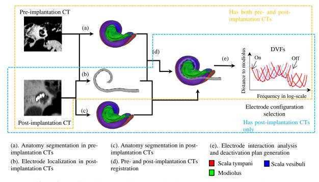
Figure 2. Workflow of Image-guided cochlear implant programming (IGCIP) techniques.
