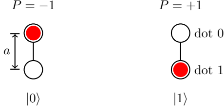
FIG. 1. Localized electronic states of a molecular double quantum dot (DQD) system provide the two classical states of a qubit. Black circles represent the two quantum dots, and a connecting bar indicates a tunneling path. A red disc represents the mobile electron.
