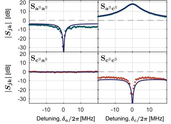
FIG. 2. Measured scattering parameters of the FPJA programmed as a phase-sensitive directional amplifier (the dots) as function of the drive detuning  $\delta_{a,c} = (\omega_{a,c}^S - \omega_{a,c})$ . The solid lines are the predictions from Eq.14. The device exhibits high gain from mode  $c$  to mode  $a$ , over a 7 MHz bandwidth, and unity transmission in the reverse direction. The device is impedance matched, with return loss exceeding 10 dB over a 4 MHz bandwidth.
