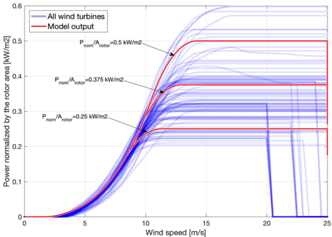
Figure 15: Comparison of all power curves contained in the database (blue curves) with the power output obtained for a power to rotor area ratio of 0.25, 0.375 and 0.5 kW/m<sup>2</sup> (red curves)
