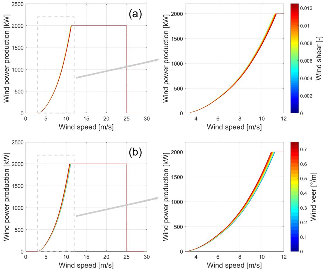
Figure 6: Influence of the wind shear (a) and the wind veer (b) on the power curve of a typical 2-MW wind turbine (80-meter rotor diameter and hub-height of 60 meters)
