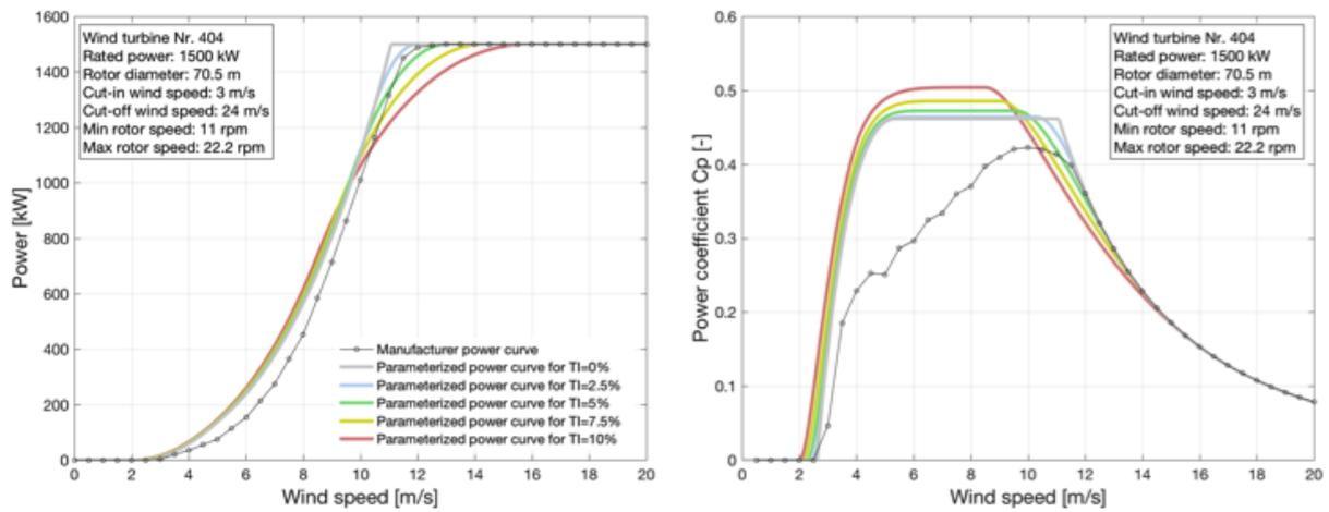
Figure 14: Comparison of the model output with the power curve of wind turbine 404 of [thewindpower.net](http://thewindpower.net) (2018), which has an unknown divergence
