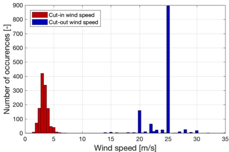
Figure 10: Distribution of the cut-off wind speed from the European dataset of [thewindpower.net](http://thewindpower.net) (2018)
