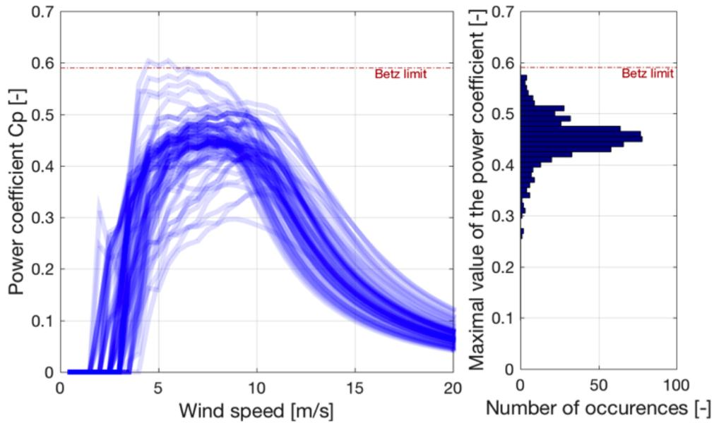
Figure 9: Left: Power coefficient as a function of the wind speed for the power curves available in [thewindpower.net](http://thewindpower.net) (2018) dataset. Right: distribution of the maximal power coefficient evaluated for all available power curves.
