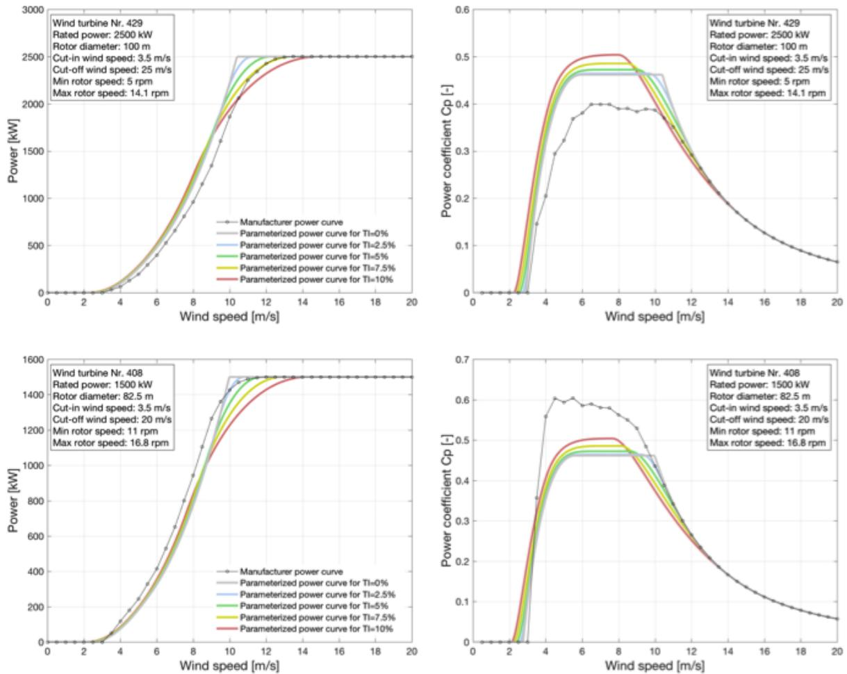
Figure 13: Comparison of the model output with the power curves of two wind turbines which are modelled with lower quality. The two rows show the wind turbines 429 and 408 of [thewindpower.net \(2018\)](#)
