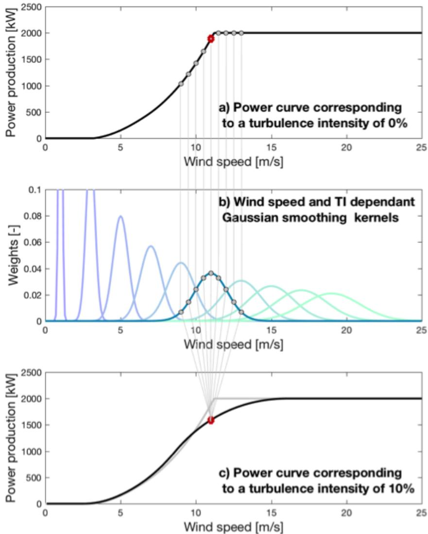
Figure 2: Illustration of the method used to calculate the effect of turbulence intensity on the power curve: the upper, middle and lower plots represent respectively the original power curve, the different Kernels and the final power curve. An example of calculation for a wind speed of 11 m/s is provided.
