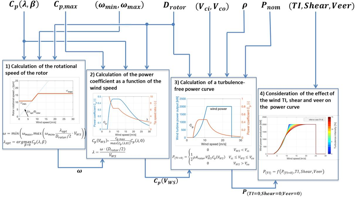
Figure 7: Flow chart representing the main computation steps for the estimation of a power curve from characteristics of a wind turbine
