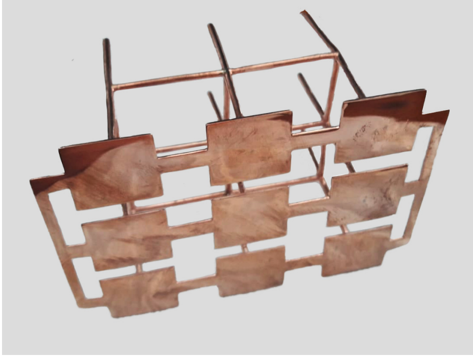
Figure 8: 10:1 scaled version of the planar metamaterial of Fig.2.
