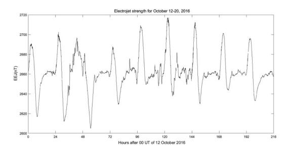
Figure 8: Electrojet strength during October 1220, 2016, taking the difference of horizontal component of the Earth's magnetic field (H in nT) of Alibag (station away from magnetic equator) from that of Dalat (a station near magnetic equator).
