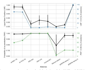
Fig. 12: Variation of the average value and standard deviation of the *LMF* and *PNP* indices for different materials and a minimum allowable thickness configuration (black lines). Percentage of solutions over a 0.9 *LMF* index (blue line) and over a 0.99 *PNP* index (green lines).
