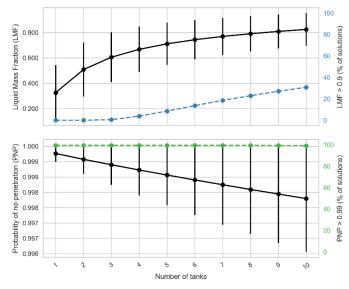
Fig. 16: Variation of the average value and standard deviation of the *LMF* and *PNP* indices for variable dimensions of stainless steel componenents (black lines). Percentage of solutions over a 0.9 *LMF* index (blue line) and over a 0.99 *PNP* index (green lines).
