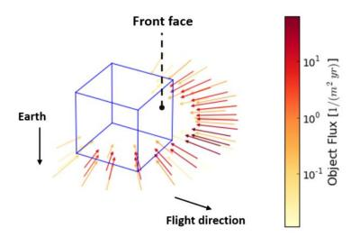
Fig. 6: Vector flux representation for the example subdivision. The colour-map represents the flux magnitude of the vectors.
