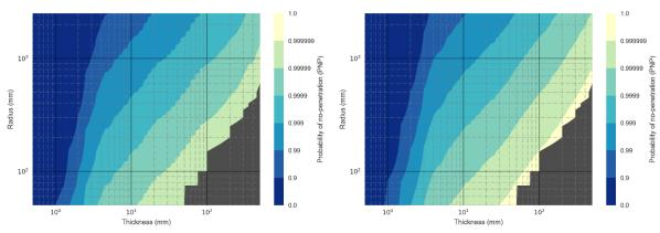
Fig. 25: Survivability contour map. Aluminium 7075-T6 Cube. Orbit 1 case on the left, Orbit 3 case on the right.
