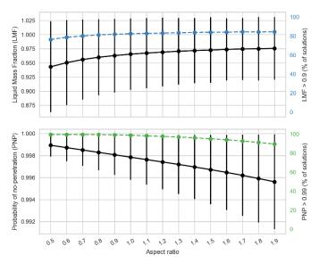
Fig. 17: Variation of the average value and standard deviation of the *LMF* and *PNP* indices with changing aspect ratio for aluminium alloy componenents (black lines). Percentage of solutions over a 0.9 *LMF* index (blue line) and over a 0.99 *PNP* index (green lines).
