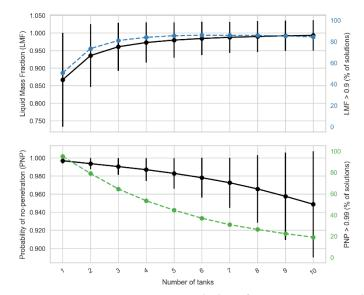
Fig. 15: Variation of the average value and standard deviation of the *LMF* and *PNP* indices for variable dimensions of aluminium alloy componenents (black lines). Percentage of solutions over a 0.9 *LMF* index (blue line) and over a 0.99 *PNP* index (green lines).
