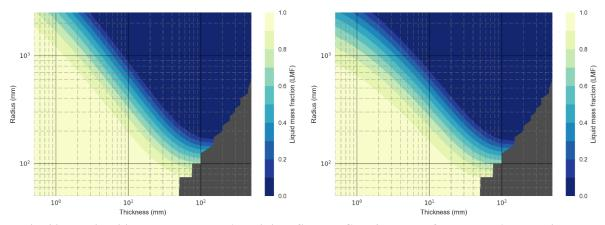
Fig. 20: Demisability contour maps. Aluminium Sphere. Case 3 on the left and case 6 on the right.
