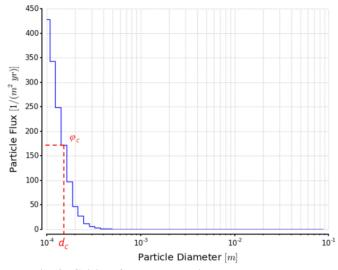
Fig. 8: Critical flux computation methodology
