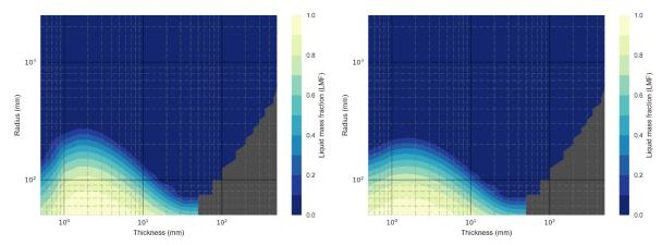
Fig. 21: Demisability contour map. Stainless Steel Sphere. Case 3 on the left and case 6 on the right.
