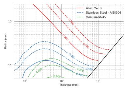
Fig. 23: Comparison between the Liquid Mass Fraction of right cylinders made of aluminium 7075-T6, stainless steel, and titanium 6AI-4V for the orbit case 1
