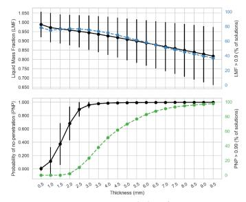
Fig. 13: Variation of the average value and standard deviation of the *LMF* and *PNP* indices for variable thicknesses of aluminium alloy componenents (black lines). Percentage of solutions over a 0.9 *LMF* index (blue line) and over a 0.99 *PNP* index (green line).
