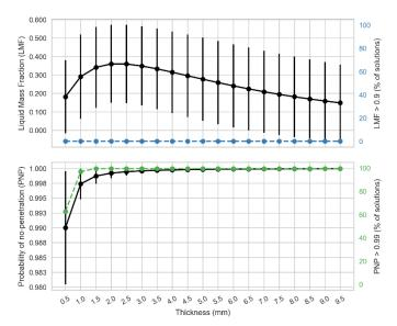
Fig. 14: Variation of the average value and standard deviation of the *LMF* and *PNP* indices for variable thicknesses of stainless steel componenents (black lines). Percentage of solutions over a 0.9 *LMF* index (blue line) and over a 0.99 *PNP* index (green line).
