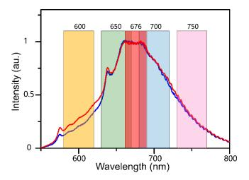
Fig. S7 Fluorescence spectrum of NV-centers situated in width-gradient circular nanoridges, further examined of wavelength dependent response in Fig. S8 top panel (blue) and lower panel (red). Transparent boxes indicate the transmission band of band-pass filters used for filtering with a center wavelength indicated above the respective boxes.
