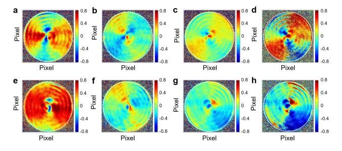
Fig. S6 Normalized Stokes parameters for many NV-centres samples. **a**,  $S'_1$ , **b**,  $S'_2$ , **c**,  $S'_3$ , and **d**,  $P_c$  for righthand width-gradient circular nanoridges. **e**,  $S'_{11}$ , **f**,  $S'_2$ , **g**,  $S'_3$ , and **h**,  $P_c$  for left-hand width-gradient circular nanoridges.
