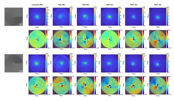
Fig. S8 Far-field intensity and normalized Stokes parameters for many NV-centres samples with different band pass filters.
