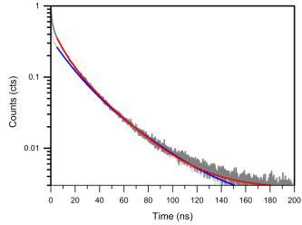
Fig. S10 Lifetime measurement of single NV-center. Experimental data is given in gray and exponential fit in blue and red, for measurement without and with width-gradient circular nanoridges respectively.
