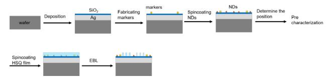
Fig. S4: Process for fabrication spinning photon sources.
