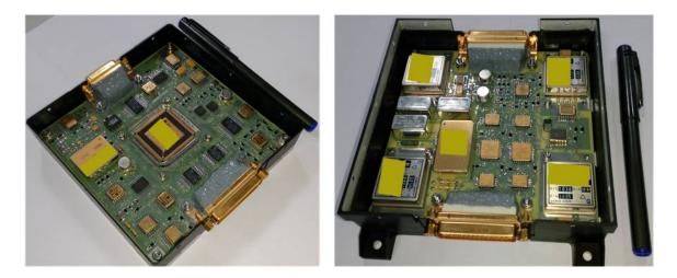
Fig. 8: FPGA PCB (left), Power PCB (right) of XSM processing electronics.
