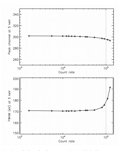
Fig. 10: Peak channel and FWHM variation with incident count rate at 5 keV. The spectral performance does not vary significantly till 1x10<sup>5</sup> counts/s.
