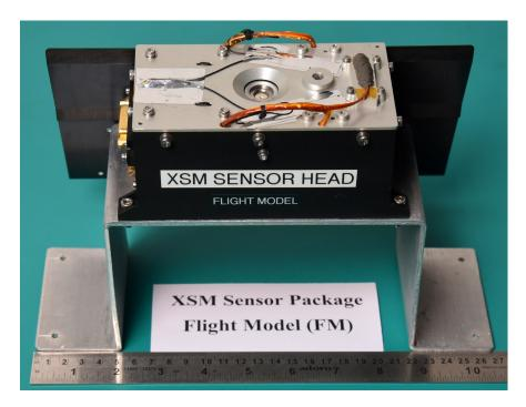
Fig. 3: XSM Sensor package Flight Model.
