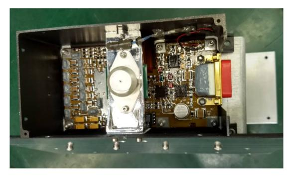
Fig. 4: XSM sensor package without mechanism.
