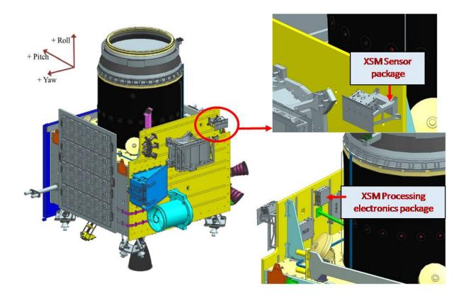
Fig. 2: Mounting locations of XSM packages on Chandrayaan-2 spacecraft.
