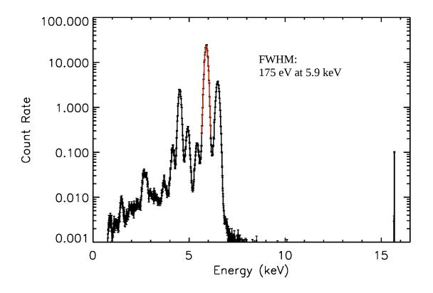
Fig. 9: XSM spectrum acquired with calibration source. Lines at 5.89, 6.49, 4.51 and 4.95 keV are prominent along with other fainter lines in the spectrum. The spectral resolution measured as FWHM of line at 5.89 keV is 175 eV.
