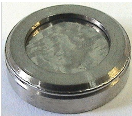
Figure 5 : Encapsulated ^{244}\text{Cm} alpha source.
