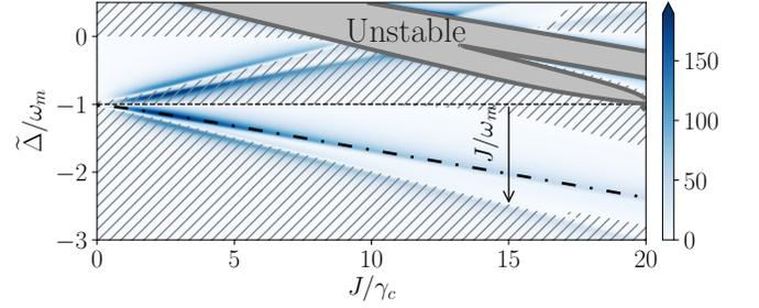
FIG. 4. Absolute value of the predicted net permanent heat current  $|Q_C|$  in units of  $\omega_m \times \gamma_m$  around a ring of cavity-coupled optomechanical resonators as a function of the inter-cavity coupling and the detuning. The hatched regions correspond to negative values. The system is unstable in the gray region.
