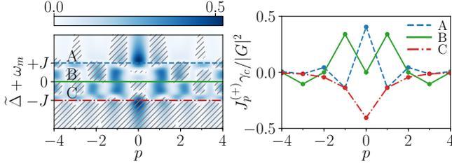
FIG. 2. Left panel: absolute value of the effective coherent coupling rate  $J_p^{(+)}$  between mechanical sites as a function of their distance  $p$  and the nonlinear detuning  $\tilde{\Delta}$ . The hatched regions correspond to negative values. Three horizontal section cuts (labeled as A, B, C) are plotted in the right panel. Here  $J/\gamma_c = 2$ .
