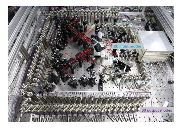
**Fig. S8:** An illustration of photonic network setup build in our laboratory. The interferometers are placed at the center of the optical table. At the right side, 20 input collimators (shown in the blue box) inject 20 beams into the photonic network. When passing through it, 60 output beams are separated by mini-mirrors to surrounding 60 collimators (shown in the purple box) to collect photons using single-mode fibers.
