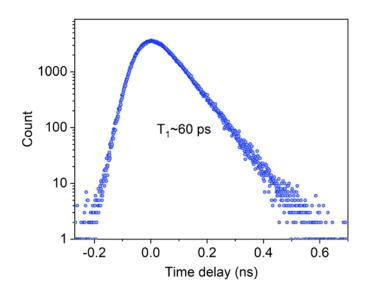
**Fig. S2:** The resonance fluorescence lifetime when the quantum dot is resonant with the micropillar cavity at ~4 K.
