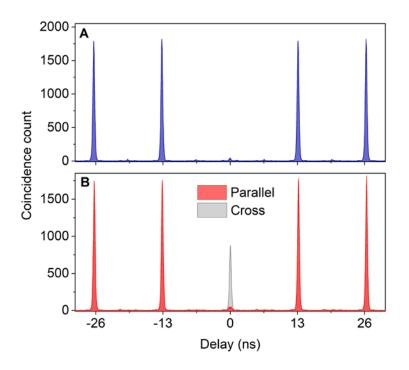
**Fig. S3:** The purity and indistinguishability of single-photon source. **A**. The second-order correlation function at zero-time delay is 0.025(1). **B**. Hong-Ou-Mandel visibility of 0.933(1) is measured with a 16-pulse emission time separation.
