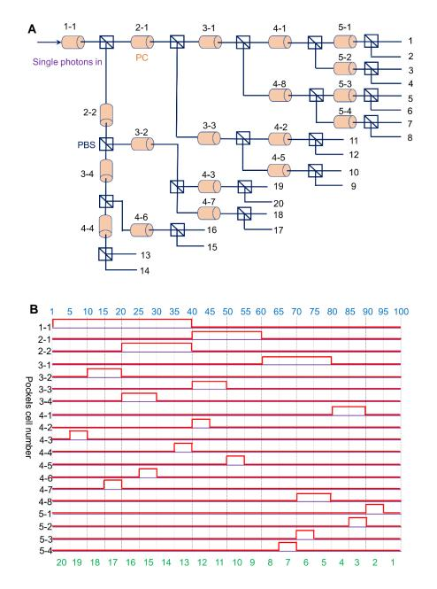
**Fig. S5: A.** The architecture of the demultiplexers used in this experiment. A stream of single photon pulses can be divided into 20 segments by 19 pairs of PC and PBS. **B.** All electric signals loaded to corresponding PCs. The width and delay for all signals must be well controlled to ensure correct operation.
