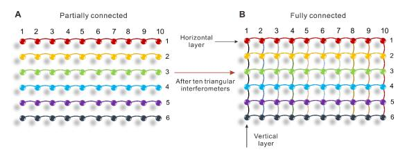
**Fig. S6:** An illustration of the interferometer. **A.** After the rectangular interferometer, all horizontal layers are connected, however, no interaction among vertical layers. **B.** After triangular interferometers, all 60 modes are fully connected.
