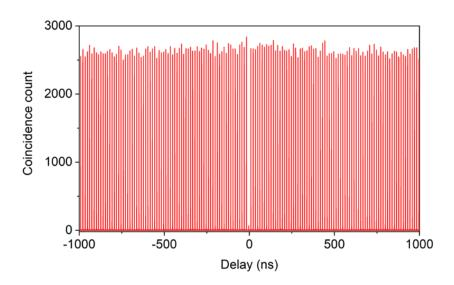
**Fig. S4:** The second-order correlation measurement at a time scale from -1000 ns to 1000 ns. The data shows that almost no blinking happens in quantum dot sample.
