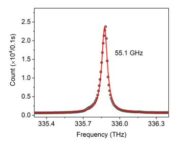
Fig. S1: The measured cavity mode of micropillar. The quality factor is ~6800.
