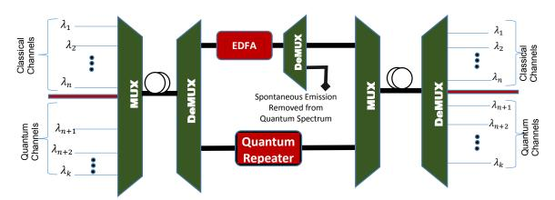
**Figure 4**: Optical communications fiber link engineered with two wavelength partitions to simultaneously carry photonic quantum states and classical traffic.
