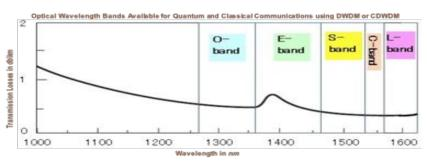
Figure 3: Optical Fiber Low Loss Transmission Spectrum
