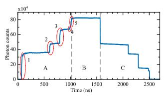
Fig. 2. Experimental data curve of FUT consisting of  $\sim$ 54 m, 20 m, 20 m and 2 m long fibers, obtained according to the output of TDC.
