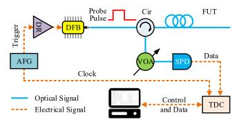
Fig. 1. Schematic of the IB-PC-OTDR. AFG: arbitrary function generator; DR: driver; DFB: distributed feed-back laser diode; FUT: fiber under test; VOA: variable optical attenuator; SPD: single photon detector; TDC: time-to-digital converter; Cir: circulator.
