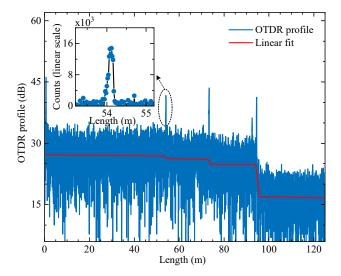
Fig. 3. OTDR trace for the FUT of about 100 m fiber. The inset shows the spatial resolution determination via the reflective peak analysis.
