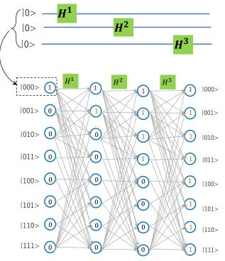
Fig. 1 Example of three gates quantum circuit and its corresponding fully connected quantum network, showing similarity to a four-layer-neural network with a equal number of nodes in the input layer, middle layer and output layer. Note that the amplitude value is not normalized for better eye-guiding illustration.
