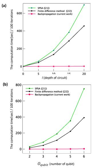
Fig. 8 Comparison of computation cost for different approaches. (a) Computation cost dependence on the depth of the quantum circuit; (b) Computation cost dependence on the number of qubits.
