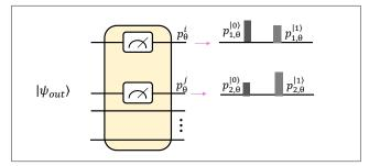
Fig. 5 Quantum circuit and measurement to obtain observation probability for classification task.
