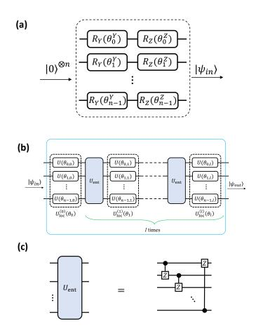
Fig. 2 (a) Preparation of input state by a unitary input gate  $U_{in}(\mathbf{x})$  exemplified by a series of rotation gates. (b) Quantum circuit to present variational parameter state  $W(\boldsymbol{\theta})$ . *l* denotes the depth of quantum circuit. (c) Quantum entanglement circuit where  $U_{ent}$  gate is composed of *CZ* gates from qubit j to qubit (j+1) mod n, j  $\in \{0, ..., n-1\}$ .
