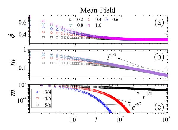
FIG. 2: Simple mean-field analysis of the system. (a): Time evolution of the entropy flux  $\phi$  for different initial magnetizations  $m_0$  indicated at criticality  $p_c = 5/6$ . (b) The corresponding time evolution of the magnetization m also at criticality. (c) Deviation from  $p = p_c$  of the magnetization m for several values of p indicated. The initial condition is  $m_0 = 1$ .
