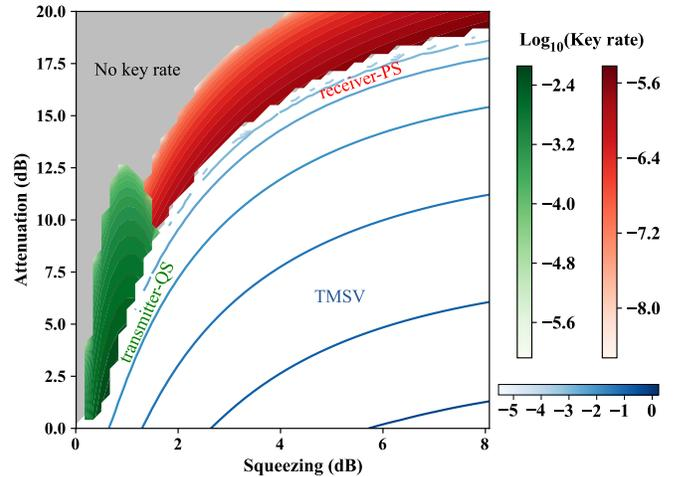
Fig. 6. Contour plots of  $\log_{10}(\text{Key rate})$  as a function of photon loss and the initial squeezing of the TMSV states. The key rate is presented in units of bit/pulse. The areas in green, red and blue represent the areas in which the highest key rates are achieved by transmitter-QS, receiver-PS and TMSV states respectively. The area in grey corresponds to the parameters for which no key rates can be obtained by any operation.
