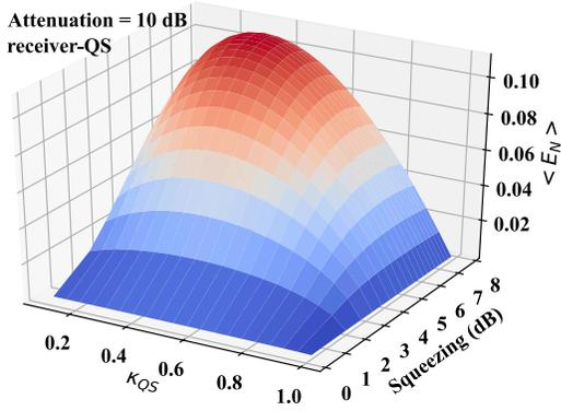
Fig. 4. The entanglement rate obtained after multiple applications of a receiver-QS, as a function of the initial squeezing of the TMSV and the parameter  $\kappa_{QS}$ . The photon loss is fixed at 10 dB.
