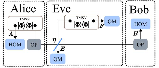
Fig. 2. The entanglement based CV-QKD protocol [14]. Alice transmits the mode  $B$  of a TMSV state to Bob. Separately, Eve prepares a TMSV state of her own, and sends mode  $E$  through a BS that mimics the channel. Afterwards, she can utilize any measurement on her modes to extract all the information possible. Here OP = QS or PS, HOM = homodyne measurement and QM = quantum measurement.
