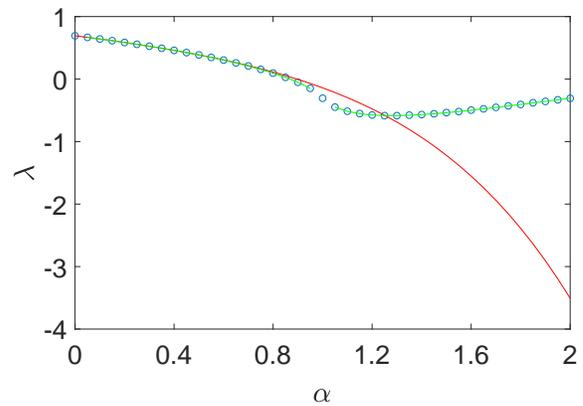
FIG. 3. (Color online) The dependence of the MLE on  $\beta$  for the system described by Eq. (32). The Monte carlo result is marked with (blue) circles while the exact one is plotted with (green) solid lines. The analytic approximation is plotted with (red) solid lines.
