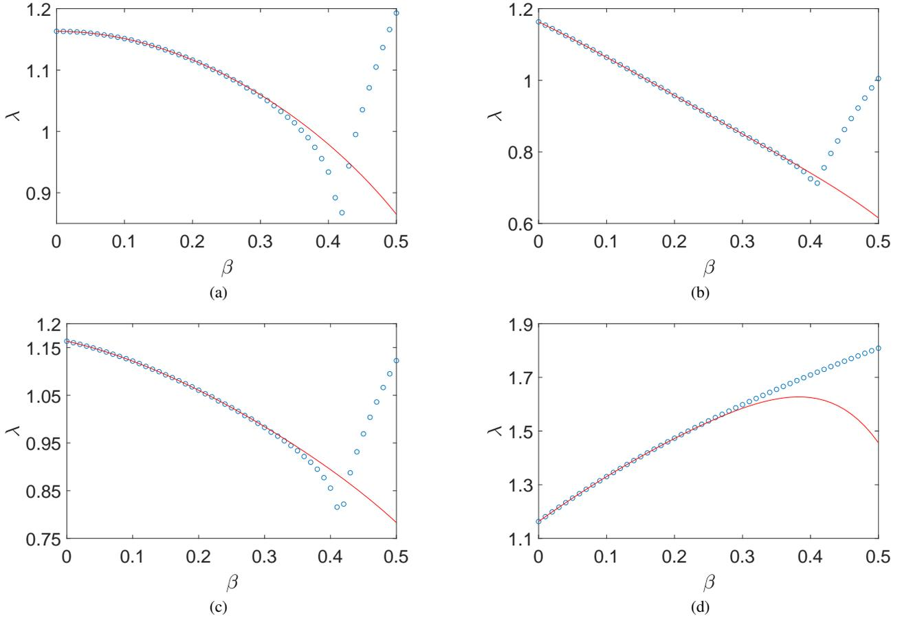
FIG. 1. (Color online) The dependence of the MLE on  $\beta$  for different probabilities  $p$  of taking the plus and minus sign in Eq. 19. (a)  $p = 0.5, 0.5$ ; (b)  $p = 0.2, 0.8$ ; (c)  $p = 0.4, 0.6$ ; (d) the result for the system in Eq. (24). The Monte carlo results are marked with (blue) circles while the analytic approximation is plotted with (red) solid lines.
