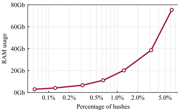
Figure 5: RAM usage when loading hashes from different fraction of the dataset. Computed on one shard.
