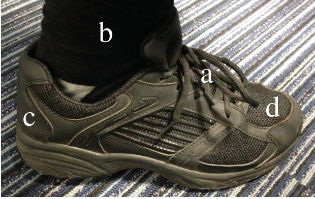
Fig. 4. Illustration of the sensor placements a) 'Shoelaces', b) 'Ankle', c) 'Heel', and d) 'Toes'.
