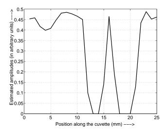
Fig. 12. The plot of the estimated amplitude vs position of the PMT along the cuvette in the case of amplitude estimated from the MLE for quantized data. The turbidity level is given by  $L/l^* = 2.14$ . The presence of the glass rod is clearly visible.
