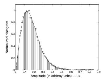
Fig. 2. The normalized histogram of the noise shows that it follows a Rayleigh distribution. The 's' parameter of the Rayleigh pdf is estimated from a best-fit curve to the above histogram.
