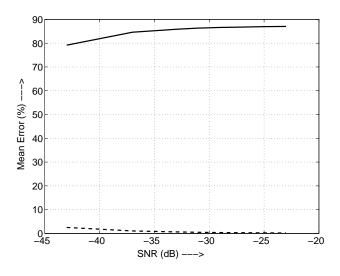
Fig. 3. A plot of the percentage error in estimated amplitude vs SNR in the input in the case of the linear estimator employing MLE. The dotted line represents the case when the frequency of the sinusoid is known exactly. The solid line is for the case when frequency is known only within an error of 0.05%.
