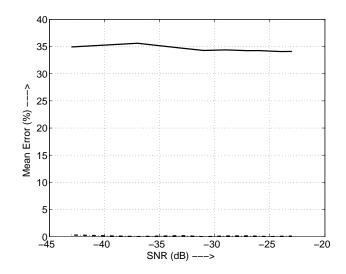
Fig. 11. The plot of the percentage error in the estimated amplitude vs SNR in the input for the method employing the MLE for quantized data. The dotted line represents the case when the frequency of the sinusoid is known exactly. The solid line is for the case when frequency is known only within an error of 0.05%.
