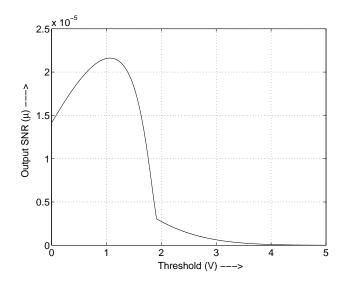
Fig. 5. Plot of equation 19 for output SNR  $\mu$  vs threshold  $\gamma$ . The maximum SNR occurs around  $\gamma = 1.064$ .
