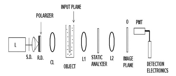
Fig. 1. The experimental setup used for Polarization Discrimination Imaging. L is the Laser, S.D. and R.D. are the static and rotating diffusers, CL is the collimating lens, L1 and L2 are the imaging lenses.
