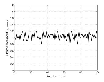
Fig. 7. Plot of the optimal threshold for the quantizer obtained for one hundred samples of the simulated data. The SNR in the data is kept at -23dB and the noise variance is kept at unity. The average value of the optimal threshold obtained is 1.046 which can be compared to the value obtained from eqn. (20) which is 1.064.
