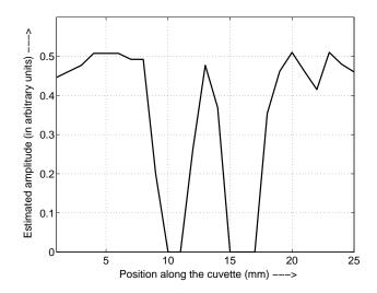
Fig. 9. The plot of the estimated amplitude vs position of the PMT along the cuvette in the case of amplitude estimated from the 3 level quantizer employing cross-over probability method. The turbidity level is given by  $L/l^* = 2.14$ . The presence of the glass rod is clearly visible.
