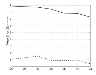
Fig. 8. The plot of the percentage error in the estimated amplitude vs SNR in the input from the 3 level quantizer employing the crossover probability method. The dotted line represents the case when the frequency of the sinusoid is known exactly. The solid line is for the case when frequency is known only within an error of 0.05%.
