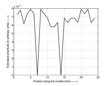
Fig. 16. The same as Figure 15 except  $L/l^* = 5.05$ . The presence of the glass rod is still clearly visible.
