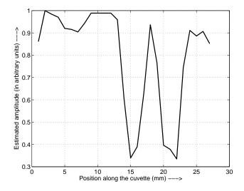
Fig. 6. The plot of the estimated amplitude vs position of the PMT along the cuvette in the case of lock-in detection. The turbidity level is given by  $L/l^* = 2.14$ . The presence of the glass rod is clearly visible.
