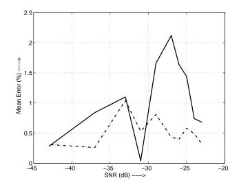
Fig. 14. The plot of the percentage error in the estimated amplitude vs SNR in the input employing the expected power of the quantized output. The dotted line represents the case when the frequency of the sinusoid is known exactly. The solid line is for the case when frequency is known only within an error of 0.05%.
