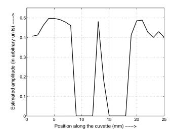
Fig. 15. The plot of the estimated amplitude vs position of the PMT along the cuvette in the case of amplitude estimated from the 3 level quantizer employing the expected power of the quantized output method . The turbidity level is given by  $L/l^* = 2.14$ . The presence of the glass rod is clearly visible.
