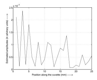
Fig. 4. The plot of the estimated amplitude vs the position of the PMT in the case of amplitudes estimated by the linear method employing MLE. The  $L/l^*$  of the turbid medium is 2.14. The pattern does not show forth the presence of the glass rod.
