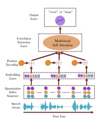
Fig. 1. Structure of Proposed Fast Correlation Extraction Model
