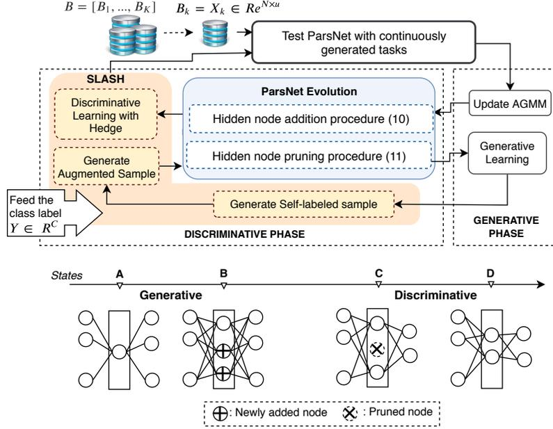
Figure 1: ParsNet learning policy and network evolution. **State A**: ParsNet starts its learning process with a hidden node in the generative phase. **State B**: Hidden nodes are added. **State C**: A hidden node is pruned on demand. **State D**: Final network structure.
