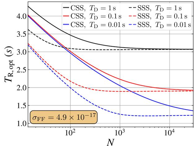
FIG. 6. Optimal Ramsey interrogation times to the results of Figure 3(a) in the main text. Based on the logic of the main text the optimal interrogation times follow the same overall trend as the instability. For the chosen laser noise parameters (see main text for details) they are all on the order of a few seconds.
