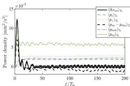
FIGURE 11. Evolution of the derivative of total energy, injected power and the different dissipative terms in time, for a linear experiment with forcing amplitude  $a_0 = 5$  mm in the 3D tank. Note the  $10^{-3}$  factor on the  $y$ -axis. The field had been filtered around the forcing frequency before computing these quantities.
