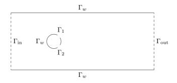
FIGURE 1. Computational domain of the cylinder wake.
