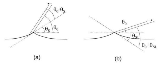
**Fig. 5:** (a) In Extrand and Kumagai point of view, the liquid can advance ahead of the contact line (before relaxation of the substrate to a new shape), when the effective contact angle  $\theta_0$ - $\theta_s$  defined with respect to the inclined dry substrate becomes larger than a reference critical value  $\theta_a^{(0)}$ . (b) A similar argument can be built for receding of the liquid, the condition becoming now  $\theta_0 + \theta_{SL} < \theta_r^{(0)}$ .
