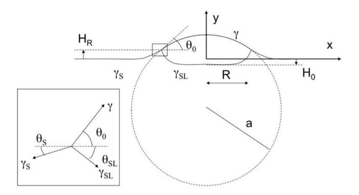
**Fig. 4:** Notations and geometry involved in the problem of a liquid ridge (or rivulet) lying one a deformable substrate.
