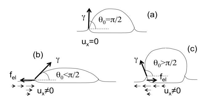
**Fig. 3:** Depending on the history of a drop, and if the interaction between the contact line and the substrate allows some possible pinning effects, different states can occur even when the "natural" contact angle should be equal to  $\pi/2$ : (a) "ideal" state, with no displacements developing in a direction parallel to the substrate, (b-c) states "under tension" in which the capillary force is balanced by elastic forces.
