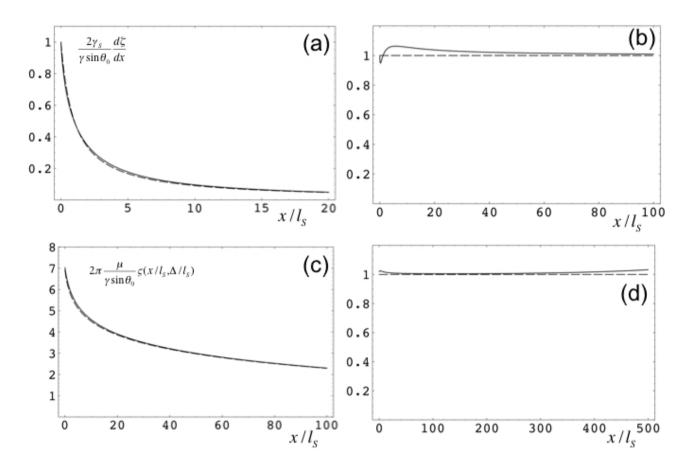
**Fig. 2**: (a) Comparison between the approximate slope distribution given by eq. 20 (dashed line) and the exact one of eq. 5 (continuous line, in the half space x>0. (b) Ratio of the exact slope distribution to the approximate one. (c) Comparison between the exact profile of the distorted surface with  $\Delta/l_s=1000$  (continuous line), to the approximate one (dashed line) with  $\Delta'/\Delta=1.7807$ . (d) ratio of the exact surface profile to the approximate one.
