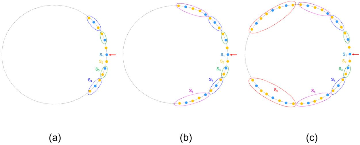
**Figure 2.** Diagram of ring of cores: 4<sup>th</sup> order FCRF4 with 13 cores (a), 5<sup>th</sup> order FCRF5 with 23 cores (b), and 6<sup>th</sup> order FCRF6 fiber with 39 cores (c). Red arrow indicates input core.
