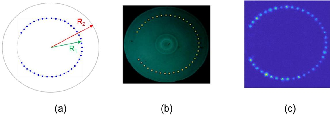
**Figure 1.** Diagram of MCRF with 39 identical SM cores (a), image of the fabricated fiber (b), and the image of the fiber that is overfilled with light of wavelength  $1.550 \mu\text{m}$ .
