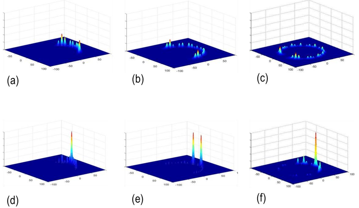
**Figure 3.** Probability distribution of photons in quantum walks: a) regular MCRF with 13 cores, b) regular MCRF with 23 cores and c) regular MCRF with 39 cores, d) FMCRF4 with 13 cores, e) FMCRF5 with 23 cores and f) FMCRF6 with 39 cores. Signal wavelength  $\lambda = 1.550 \mu\text{m}$ .
