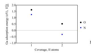
Fig. S10: Plot of adsorption energies for a single Ga atom,  $E_{ads}^{Ga}$ , as a function of the number of adsorbed surface O or N on the (2×1) reconstructed Si (001) surface supercell shown in Fig. S7. Positive (negative) energies are repulsive (attractive). Black dots and blue squares correspond to O and N atoms, respectively.
