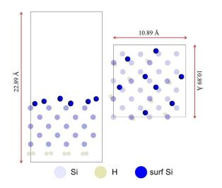
Fig. S7: Side and top views of the  $(2\times1)$  reconstructed Si (001) supercell with 8 surface Si atoms (Dark blue dots labeled as "surf Si"). The bottom surface is saturated by H atoms. By fixing the bottom 3 layers and relaxing atoms in the top 3 layers, the free (001) Si surface undergoes a reconstruction where two near surface Si atoms always come close to each other. The energy of this configuration is  $E_{Si}$ .
