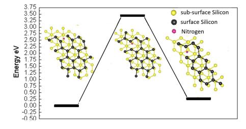
**Fig. S6:** Reaction path for N adatom (pink) diffusion on Si (111) surface viewed from the top, overlaid on a plot of the energies of the initial, intermediate, and final states. The initial energy state is defined as zero and the surface oxygen, surface silicon, and sub-surface Si are shown in green, black, and yellow, respectively.
