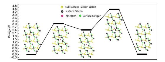
**Fig. S4:** Reaction path for N adatom (pink) diffusion on  $SiO_2(001)$  surface viewed from the top, overlaid on a plot of the energies of the initial, several intermediate, and final states. The initial energy state is defined as zero and the surface oxygen, surface silicon, and sub-surface  $SiO_2$  are shown in green, black, and yellow, respectively.
