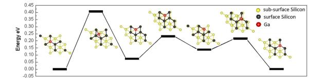
**Fig. S3:** Reaction path for Ga adatom (red) diffusion on Si (111) surface viewed from the top, overlaid on a plot of the energies of the initial, various intermediate, and final states. The initial energy state is defined as zero and the surface oxygen, surface silicon, and sub-surface Si are shown in green, black, and yellow, respectively.
