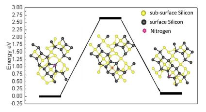
**Fig. S5:** Reaction path for N adatom (pink) diffusion on Si (001) surface viewed from the top, overlaid on a plot of the energies of the initial, intermediate, and final states. The initial energy state is defined as zero and the surface oxygen, surface silicon, and sub-surface Si are shown in green, black, and yellow, respectively.
