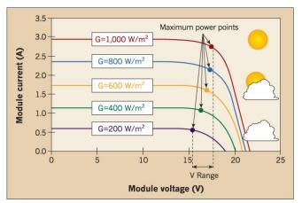
Fig.2. IV characteristic of a PV module (source: www.ecmweb.com)
