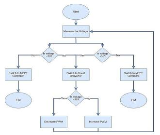
Fig.4. Flowchart of the Power Management System
