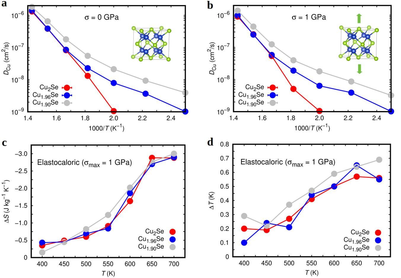
FIG. 4. Elastocaloric effects in bulk  $\text{Cu}_{2-x}\text{Se}$  at temperatures  $400 \leq T \leq 700$  K. **a** Ionic diffusion coefficients calculated at zero uniaxial tensile stress and **b**  $\sigma = 1$  GPa. **c** Isothermal entropy changes induced by a maximum uniaxial tensile stress of 1 GPa. **d** Adiabatic temperature changes induced by a maximum uniaxial tensile stress of 1 GPa.
