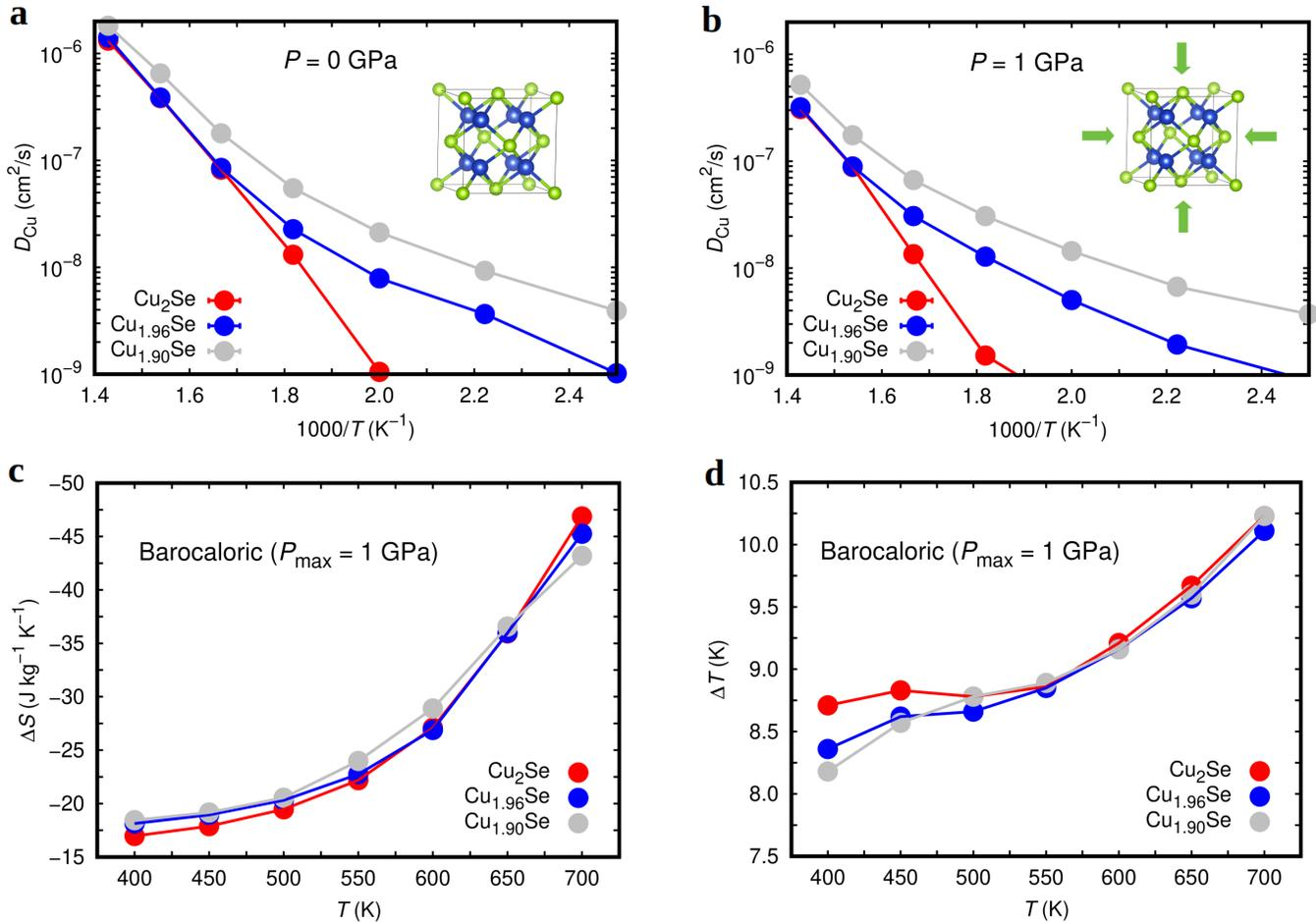
FIG. 2. Barocaloric effects in bulk  $\text{Cu}_{2-\delta}\text{Se}$  at temperatures  $400 \leq T \leq 700$  K. **a** Ionic diffusion coefficients calculated at zero pressure and **b**  $P = 1$  GPa. **c** Isothermal entropy changes induced by a maximum hydrostatic pressure of 1 GPa. **d** Adiabatic temperature changes induced by a maximum hydrostatic pressure of 1 GPa.
