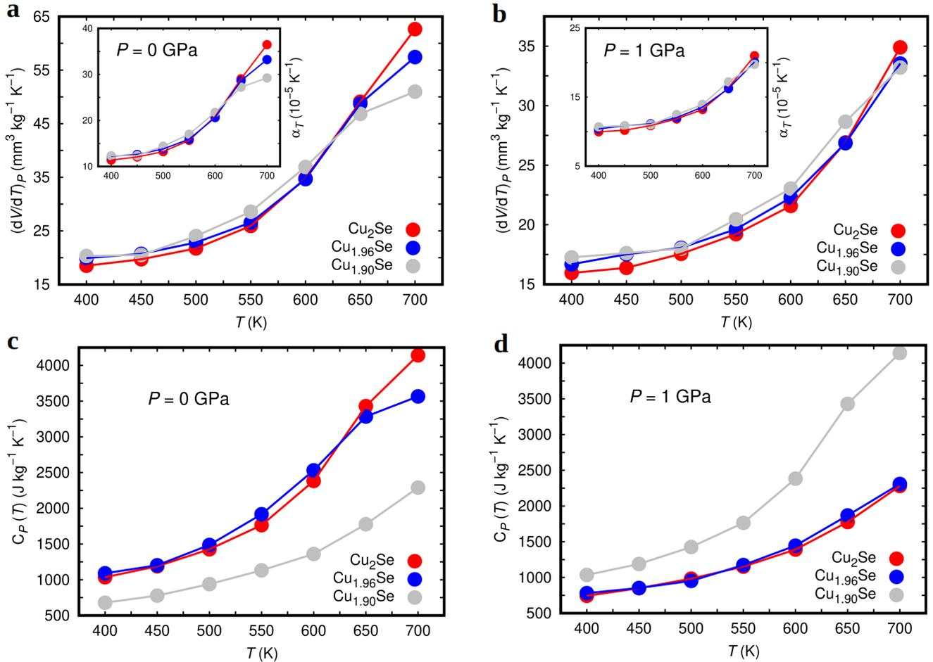
FIG. 3. Thermodynamic properties of  $\text{Cu}_{2-\delta}\text{Se}$  at temperatures  $400 \leq T \leq 700$  K. **a**  $T$ -derivative of the volume calculated at zero pressure and **b**  $P = 1$  GPa. Thermal expansion coefficients defined as  $\alpha_T = \frac{1}{V} \left( \frac{dV}{dT} \right)_P$  are shown in the insets. **c** Heat capacity calculated at zero pressure and **d**  $P = 1$  GPa.
