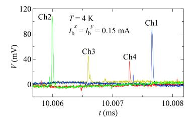
**Figure 2.** Typical signal quartet from Ch1, Ch2, Ch3, and Ch4 at T = 4.0 K with a bias current of  $I_{\rm b}^x = I_{\rm b}^y = 0.15$  mA. Notably, the negative signals from Ch1 and Ch3 are inverted by the low-noise differential amplifier. Pulsed neutrons are generated at t = 0 ms of the horizontal axis. The four signals are simultaneously generated by a single nuclear reaction event. We can find the time and coordinate of the event occurrence from the timestamps of these signals.
