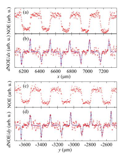
**Figure 5.** (a) Number of events (NOE) on the <sup>10</sup>B-dots boundary in the X-direction along the line  $y = 1885.5 \,\mu\text{m}$ . (b) Numerical differentiation of the NOE as a function of y with the least-squares fit line to a Gaussian function. (c) NOE on the <sup>10</sup>B-dots boundary in the Y-direction along line  $x = 6229.5 \,\mu\text{m}$ . (d) Numerical differentiation of the NOE as a function of y with the least-squares fit line to a Gaussian function.
