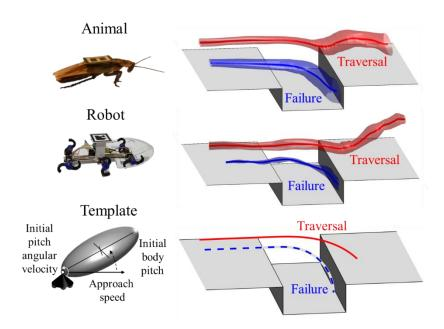
**Figure 7.** Summary of animal, robot, and template body dynamics and body-terrain interaction. Red and blue tubes and curves represent means  $\pm 1$  s.d. of vertical and lateral position of the head as the body moved forward towards the gap. The trajectories of successful traversal and failure are slightly offset in the *y*-direction for clarity. For simplicity, only movement perpendicular to the gap (within the *x-z* plane) is shown.
