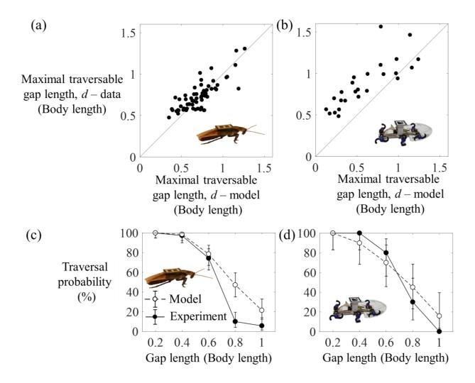
**Figure 5.** The template well predicted dynamic gap traversal. (a, b) Comparison of maximal traversable gap length measured from the infinite length gap experiment with that predicted from the model. The black diagonal line indicates perfect match between data and model. (c, d), Comparison of experimental (filled circles, solid curve) and model-predicted (open circles, dashed curve) traversal probability. Error bars represent 95% confidence interval.
