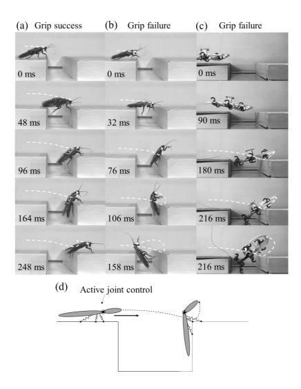
**Figure 9.** Traversal often required gripping and body flexion. (a) Successful leg gripping aided by body flexion by the animal when dynamically traversing a large gap. (b) Grip failure of the animal. (c) Grip failure of the robot. (d) A proposed two-link anchor model for dynamic gap traversal with active body flexion and leg gripping.
