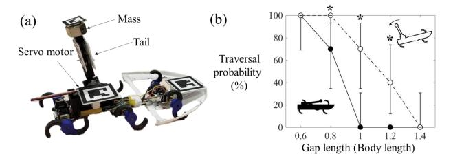
**Figure 8.** Tailed robot experiments to demonstrate the novel control strategy for dynamic gap traversal. (a) The robot with an active tail. (b) Gap traversal probability for the tailed robot with (open circles) and without (filled circles) tail actuation while running at the same speed of  $190 \pm 20 \text{ cm s}^{-1}$ .
