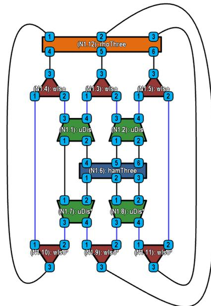
FIG. 4. One of the networks in the example project “binaryMERA.ttp” included with *TensorTrace*, which can be exported to produce the code required to optimize a binary MERA for the ground state of a 1D quantum system.
