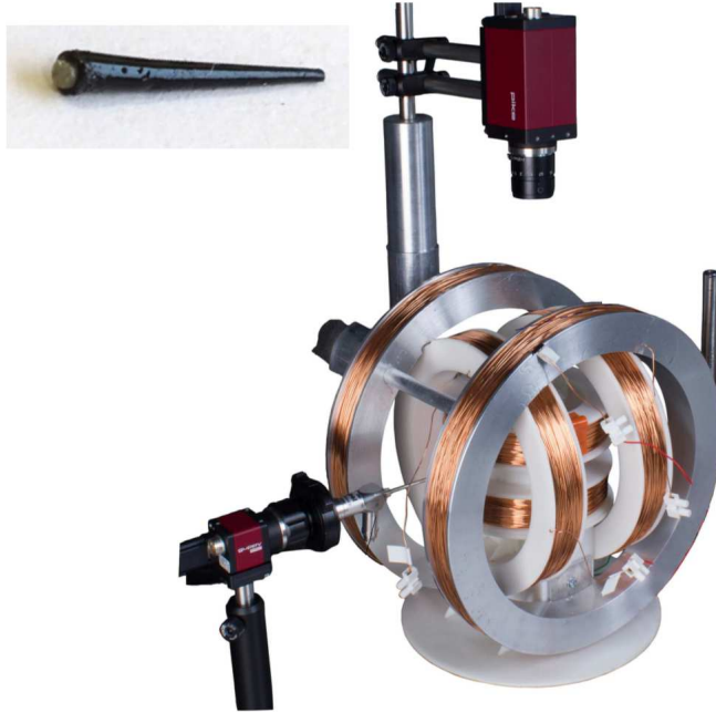
Fig. 1. Experimental setup ([21]). The three orthogonal Helmholtz coils generate a homogeneous magnetic field in the center, where the swimmer has been placed. The swimmer is tracked using two perpendicular cameras. Shown in the corner : Scaled-up flexible magnetic swimmer used in the experiments. The tail is made of an elastomer shaped by a 3D-printed mold. The head is a magnetic disk.
