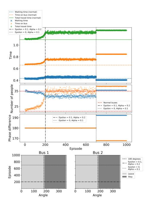
FIG. 7. Two buses with frequency detuning serving a loop of bus stops during a lull period learn the holding strategy by reinforcement learning. It is able to slightly improve the average waiting time, at the expense of slowing down the fast bus such that the average time spent on bus and average total travel time are increased.
