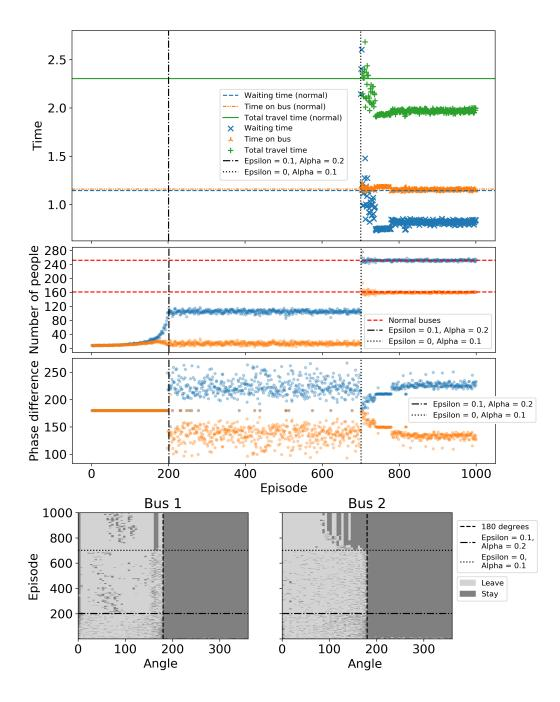
FIG. 3. Two buses with frequency detuning serving a loop of bus stops during a busy period learn the no-boarding strategy by reinforcement learning. The results are qualitatively similar to those in Fig. 2.
