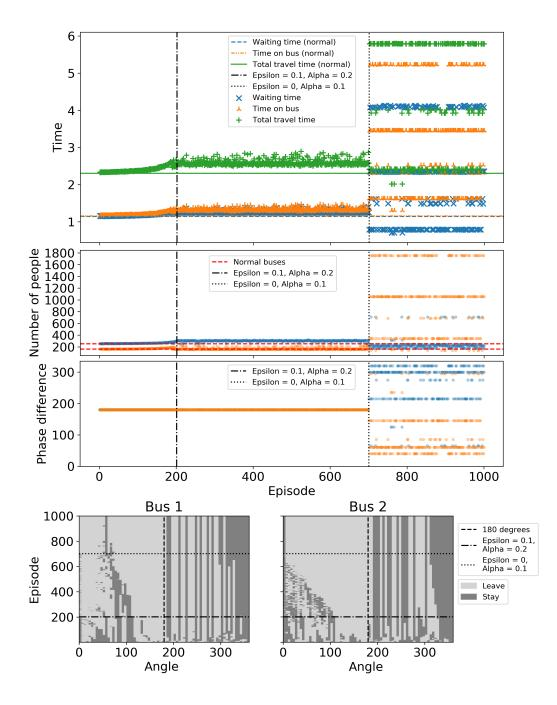
FIG. 6. Two buses with frequency detuning serving a loop of bus stops during a busy period learn the holding strategy by reinforcement learning. The entire system is slowed down greatly and generally performs worse than normal buses.
