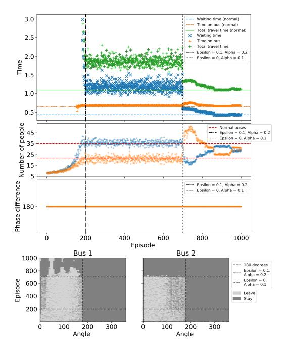
FIG. 4. Two buses with frequency detuning serving a loop of bus stops during a lull period *does* not learn the expected no-boarding strategy by reinforcement learning.
