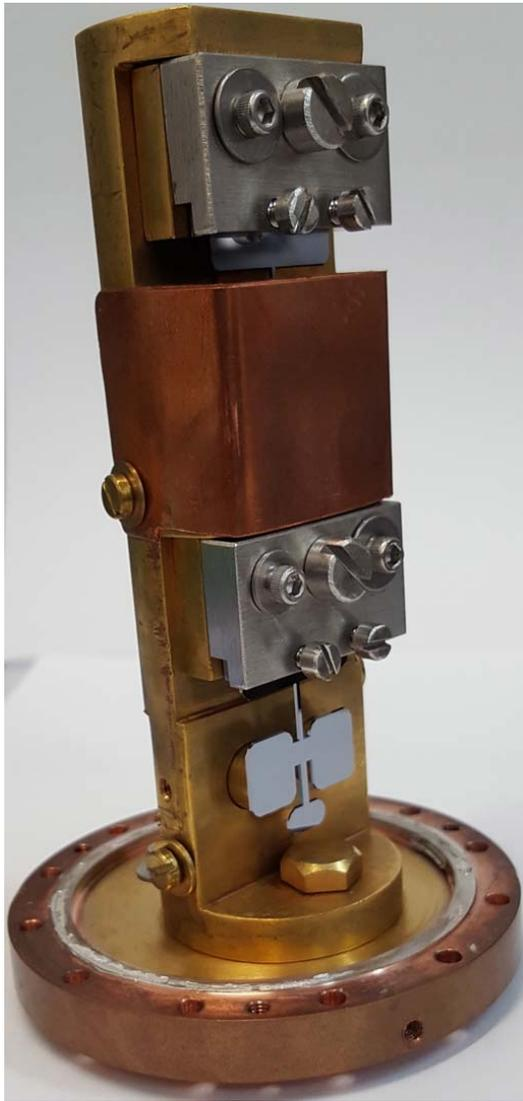
Figure 2: The gold plated copper support structure of the mechanical resonator samples is screwed to the gold plated top surface of the bottom flange of the hermetic cell. The copper sheet in front of the upper mechanical resonator protects this fragile device from breakage during assembly of the cell. Another sheet that protects the lower mechanical resonator has been removed for the photo.
