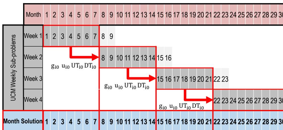
**Figure 2.** The rolling horizon simulation scheme for the unit commitment model.
