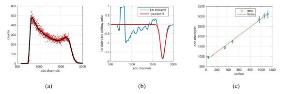
**Figure 3.** (a) The experimental spectrum recorded with a <sup>137</sup>Cs source (red dots) and the smoothed spectrum (black line). (b) The first derivative of the smoothed spectrum and the Gaussian distribution at the region of interest. (c) The calibration line which relates the deposited electron energy in the plastic scinitllator to adc channels.
