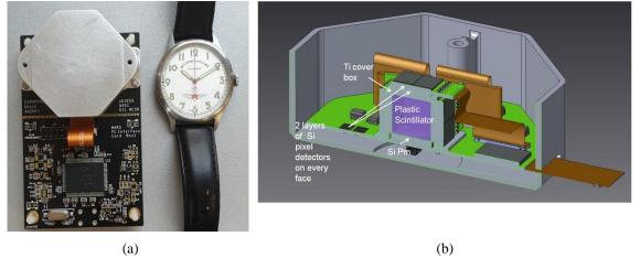
**Figure 1.** (a) The first prototype of the detecting head mounted on a custom data acquisition board. (b) Cross section view of the conceptual design of the second prototype.
