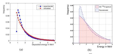
**Figure 4.** (a) The experimental energy deposition spectrum from the  $^{252}$ Cf neutron source compared to the simulated one. (b) The reconstructed neutron energy spectrum.
