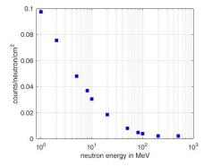
Figure 5. Simulated efficiency of the neutron detector
