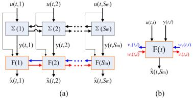
FIGURE 1. Schematic diagram of Andrea model in one dimension; (a) Overall diagram; (b) Local diagram of sub-filter
