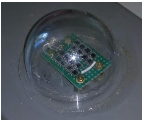
Figure 4 – Matrix of 4x4 BPW34 photodiodes
