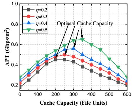
Fig. 5: APT under different cache capacities( $\gamma_0$  is 10dB)
