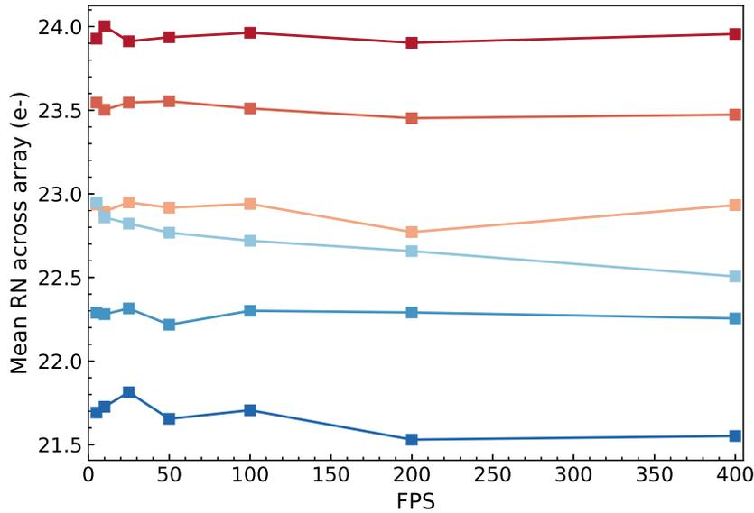
**Fig 3** Average single read CDS read noise [ $e^-$ ] across the C-RED 2 detector at different framerates and temperatures. Each data point is the average noise from 10 bias images at  $t_{\text{int}} = 20 \mu\text{s}$ . The lowest noise is  $21.6 e^-$  at FPS = 400 and  $T = -40^\circ\text{C}$ .
