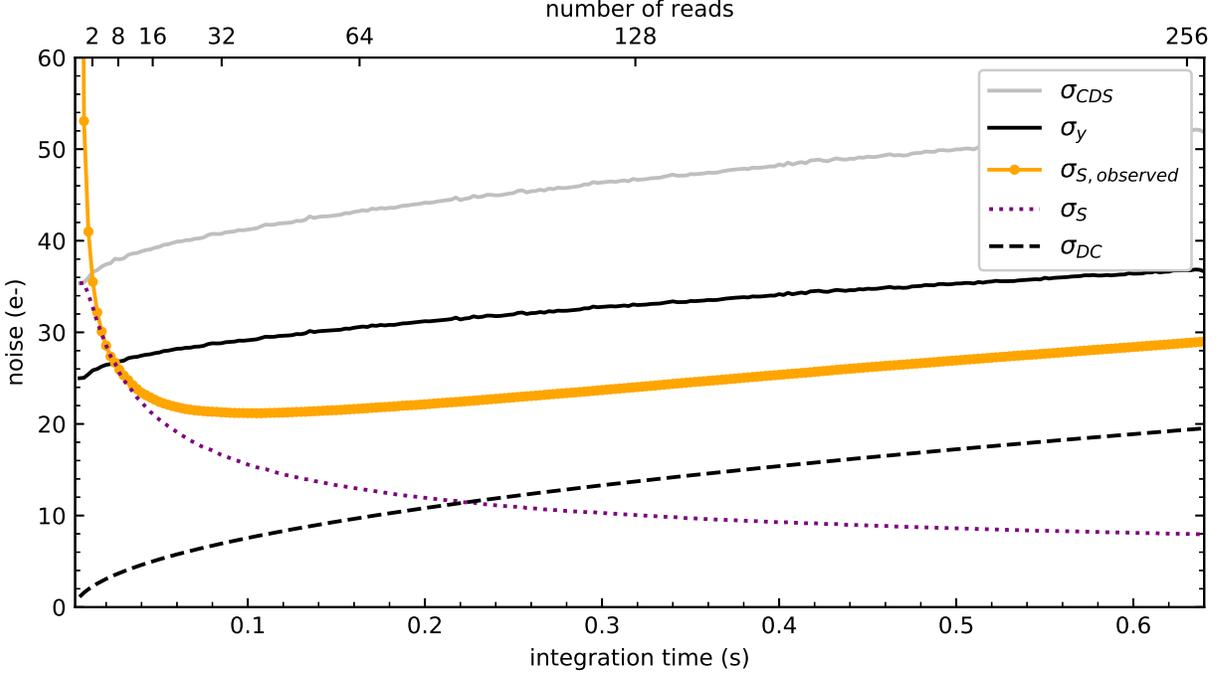
**Fig 7** The theoretical noise of an image created with multiple non-destructive reads (dotted purple) as a function of image exposure time. The theoretical values are based on the average readout noise of the individual frames (solid black). The noise of the calculated slope images is shown in orange. Also plotted is the CDS noise for comparison (solid gray) and shot noise from the dark current and background photons (dashed black).
