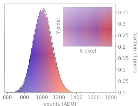
**Fig 1** An average of 10 full array bias images (insert) taken at 400 FPS,  $-40^\circ\text{C}$  and a histogram of the fraction of pixels at any given count value. A Gaussian centered on 1011 ADU and standard deviation 108 ADU is plotted on top of the histogram (black dashed line). The colors in the image correspond to the count number in the histogram. The counts range from 571 to 1850 ADU.
