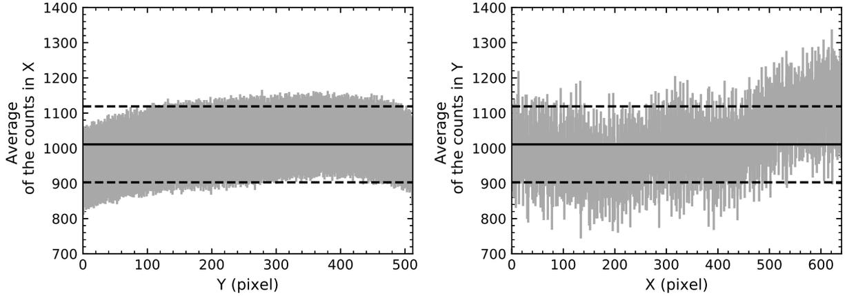
**Fig 2** Average and standard deviation of each pixel in rows Y (top) and columns X (bottom) in a bias image. Plotted in black is the average counts (solid) plus and minus one standard deviation (dashed) for the entire detector ( $\mu = 1011$  ADU and  $\sigma = 108$  ADU).
