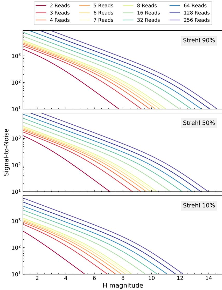
**Fig 8** Signal-to-noise expected as a function of target star magnitude at Strehl ratios of 90, 50, and 10%. The SNR calculation includes shot noise, dark current plus background black body radiation, and read noise characterized in this work. Each line is the SNR calculated using multiple non-destructive reads collected in IMRO mode.
