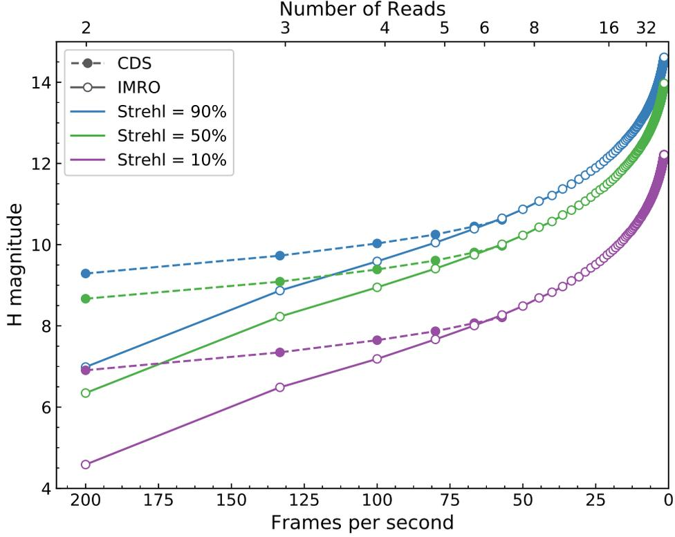
**Fig 9** Number of reads in IMRO mode (open circles), or framerate in CDS mode (filled circles) required to achieve a signal-to-noise of 10 for a given H magnitude at Strehls of 90, 50, and 10%. This requires the camera to operate at 400 FPS in IMRO mode, and in both IMRO and CDS modes the detector is operating at  $-40^{\circ}$  C.
