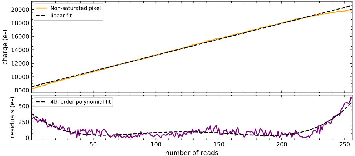
**Fig 4** *Top*: The detector response (solid orange) and linear fit to the charge accumulation (dashed black) versus number of reads. *Bottom*: Residuals between charge accumulation and linear fit (solid purple) and a 4th order polynomial fit to the residuals (black dashed). The RMS of the residuals to the polynomial fit is  $0.738 e^-$ . The configurations for this exposure were FPS = 400, T =  $-40^\circ\text{C}$ , full frame, evenly illuminated detector.
