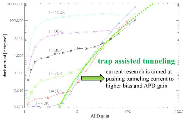
Fig. 5. Image courtesy of Leonardo MW [1]. Recent dark current measurements by ESO [2] and UH [4] for SAPHIRA ‘Mk 13/14’ devices show very low values at low temperatures and unity gain. The increase in noise with avalanche gain may limit exposure times at high gains, and is the subject of ongoing research.
