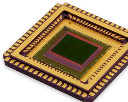
Fig. 1. Image courtesy of Leonardo MW. The SAPHIRA is a 320×256 pixel linear-mode avalanche photodiode array capable of ‘noiseless’ readouts via an upstream signal multiplication of several hundred.
