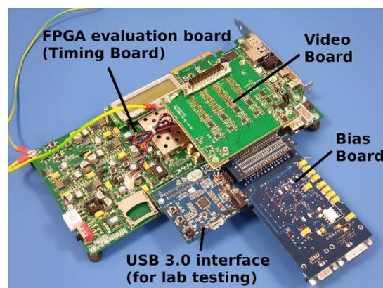
Fig. 9. Prototype Emu readout electronics, including a commercial FPGA evaluation board, one of two 16-channel ‘video boards’ for analog-to-digital conversion, and a ‘bias board’ for detector biases and clock conditioning.
