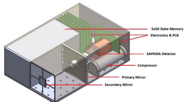
Fig. 7. Conceptual design of the 6U ‘Emu’ payload, featuring a SAPHIRA LmAPD array and ANU readout electronics. Note that the payload will in fact point ‘up’ to zenith.
