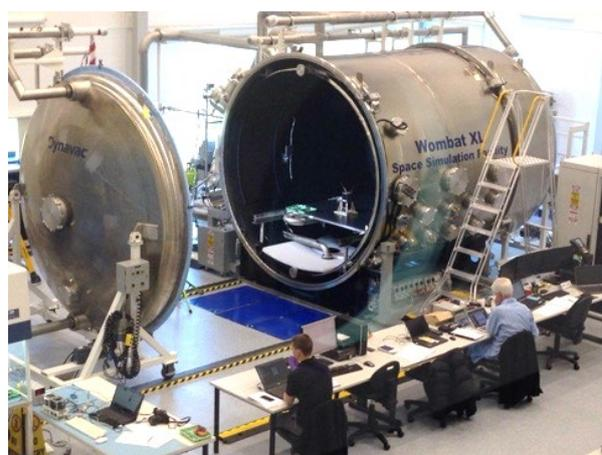
Fig. 8. Australia’s National Space Test Facility at ANU provides spacecraft qualification and test services including thermal cycling, thermal vacuum, and launch vibrations.
