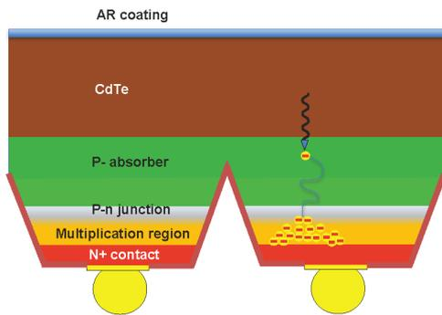
Fig. 2. Image courtesy of Leonardo MW [1]. Current-generation SAPHIRA devices use bandgap engineering and MOVPE technology to achieve linear-mode electron avalanche multiplication of several hundred times, while suppressing dark current at high gains.
