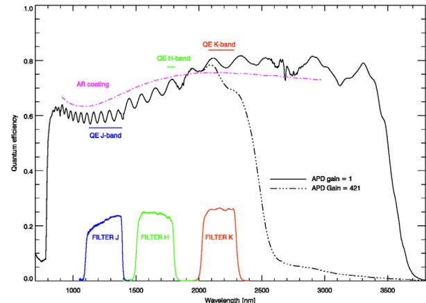
Fig. 6. Image courtesy of ESO [2]. Measured sensitivity (‘quantum efficiency’) of a SAPHIRA ‘Mk 14’ detector at unity and high (421×) gain. The response beyond 2.5–3.5  $\mu\text{m}$  photons experience only a fraction of the avalanche multiplication. The high-gain curve has been normalized.
