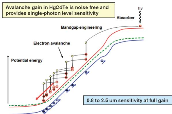
Fig. 3. Image courtesy of Leonardo MW [1]. Photons with wavelengths 0.8–2.5  $\mu\text{m}$  produce electrons in the absorber layer just like a traditional HgCdTe detector, but these electrons are then multiplied within the biased ‘multiplication region’, boosting signal levels without introducing significant excess noise [2].
