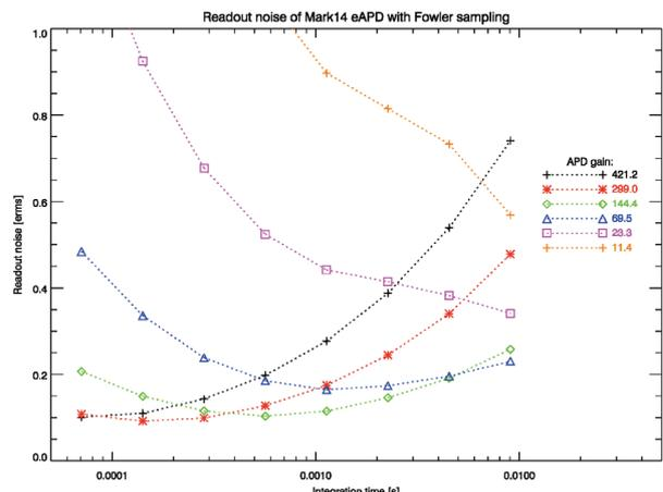
Fig. 4. Image courtesy of ESO [2]. Effective SAPHIRA readout noise values of  $<0.2 e^-$  have been demonstrated for high gains. This data used increased frame averaging for longer exposures, hence the reduction in noise for longer exposures at low gains. The increase in noise with exposure time for high gains is due to dark current (since improved).
