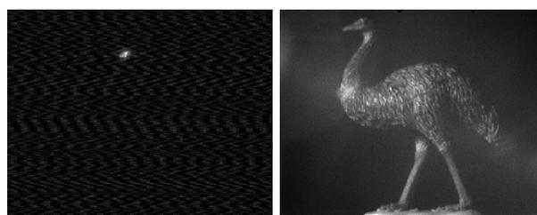
Fig. 10. The prototype readout electronics system in Fig. 9 has been tested with a SAPHIRA detector on-sky (star in H-band, left) for ‘Lucky Imaging’ at the ANU 2.3 m telescope (Siding Spring Observatory), and recently in the lab (plastic Emu in H-band, right) with improved noise performance.
