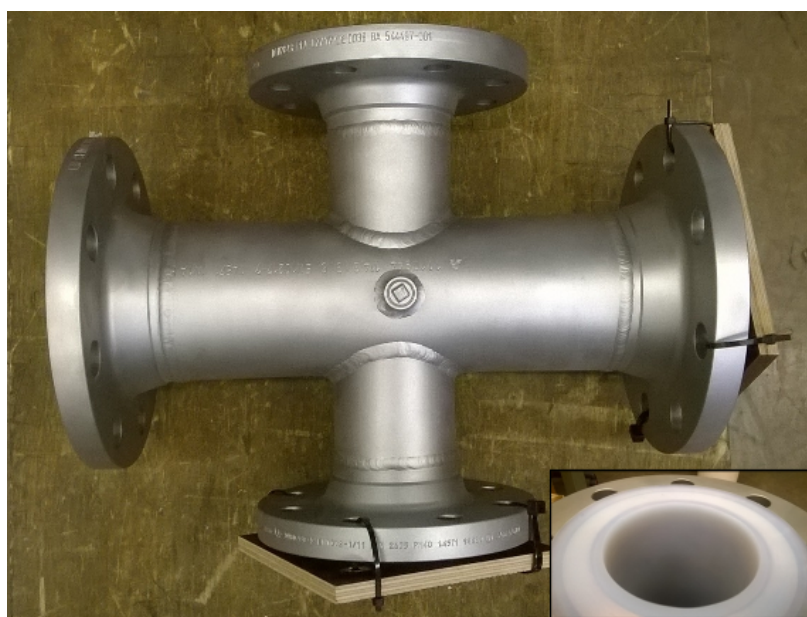
Figure 3.10.: Chemical industry standard double-tee piping lined with 4 mm PFA. The lining's theoretical, integrated dielectric strength is 320 kV. The hull is made from high grade stainless steel and rated for 25 bar overpressure.
