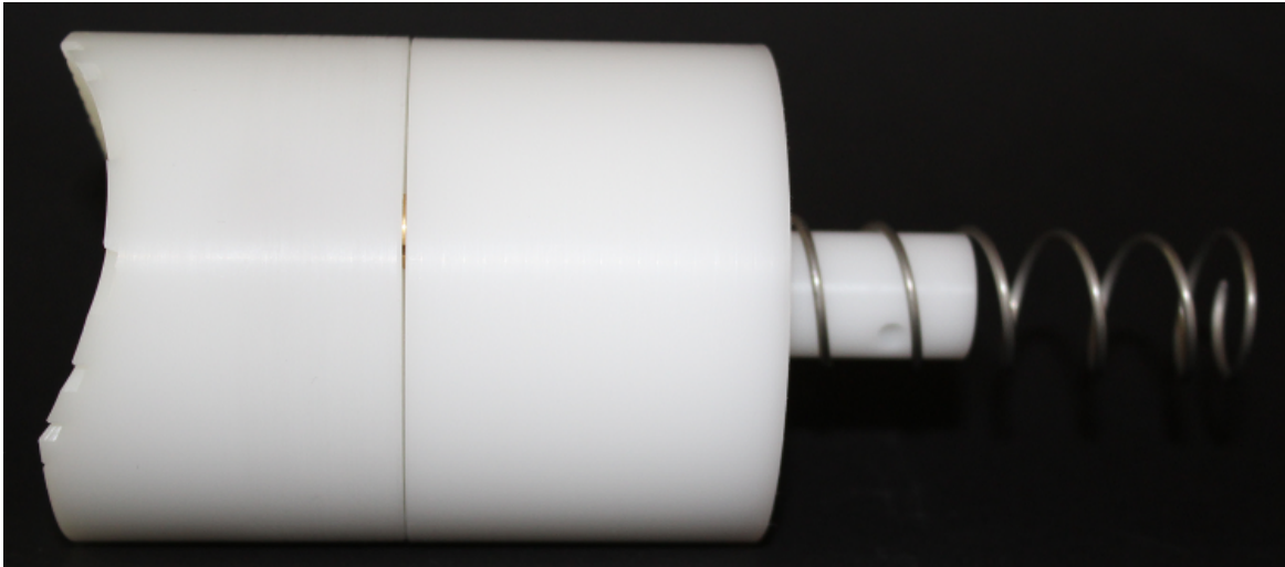
Figure A.2.: Fully assembled POM block holding the \text{Sr}^{90} sources inside. A spring pushes the block into place. The field cage is attached from the left.
