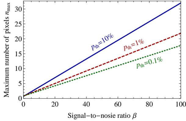
Fig. 5. Maximum pixel number as a function of the signal-to-noise ratio parameter  $\beta$ . Each line indicates the detector quality that must be achieved in order to reach a particular error threshold.
