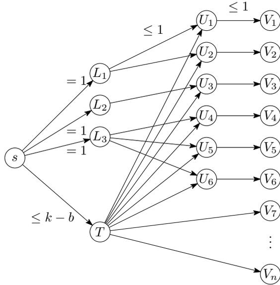
Figure 2: Part of the modified network for a solution  $T$  which is specified by  $b = 3$  sets  $L_1 = \{1, 2\}$ ,  $L_2 = \{3\}$ , and  $L_3 = \{4, 5, 6\}$ .
