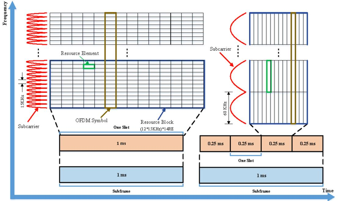
Figure 1: 5G NR Resource Grid for numerologies with sub-carriers of 15 KHz and 60 KHz
