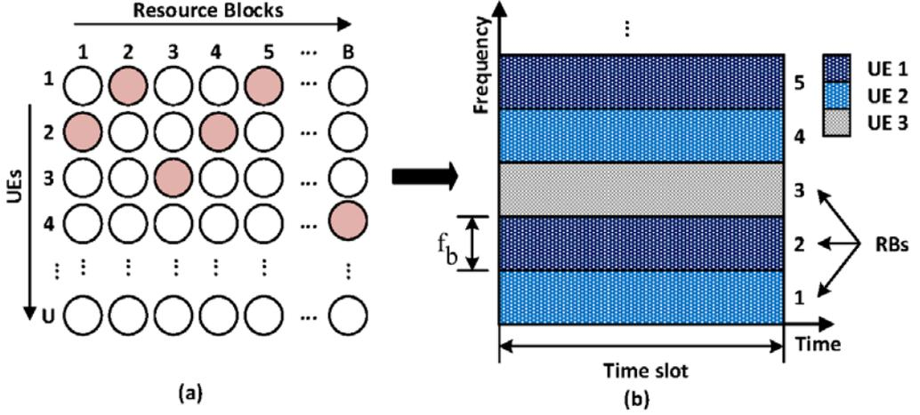
Figure 2: The relation between firing pattern of neural network and RBs allocation
