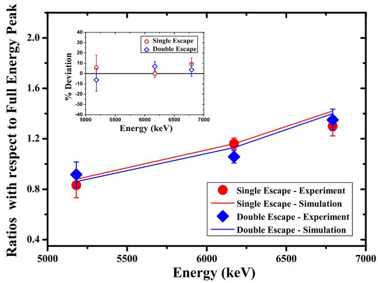
Figure 5: The relative contribution for S.E. and D.E. with respect to F.E. as a function of  $\gamma$ - energy for the BEGe detector. The percentage deviation of the experimental value from simulation is shown in the in-set figure.
