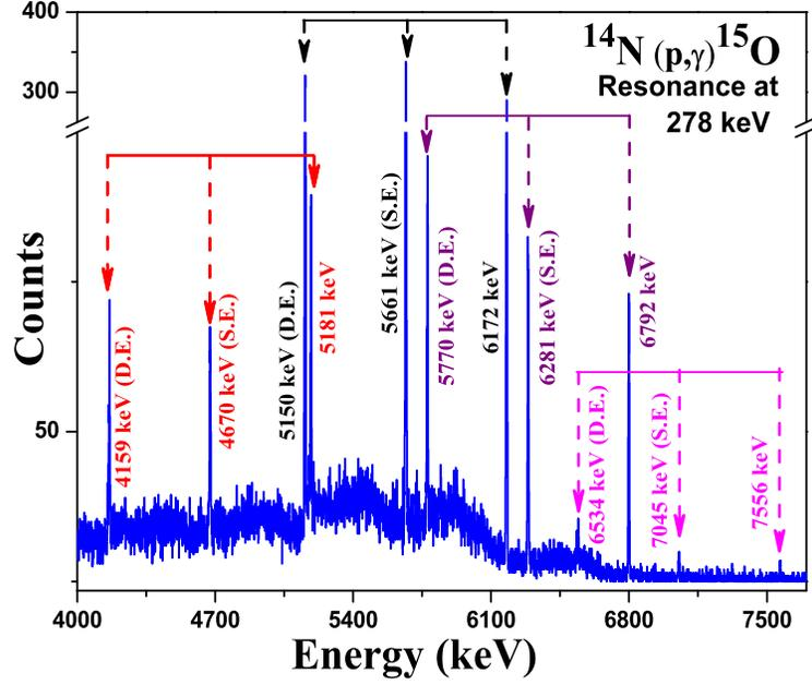
Figure 4: Typical high-energy part of  $\gamma$ -ray spectra from  $^{14}\text{N}(p,\gamma)^{15}\text{O}$  resonance reaction at  $E_p^{\text{lab}} = 278$  keV. S.E. and D.E. denote single escape and double escape peaks, respectively.
