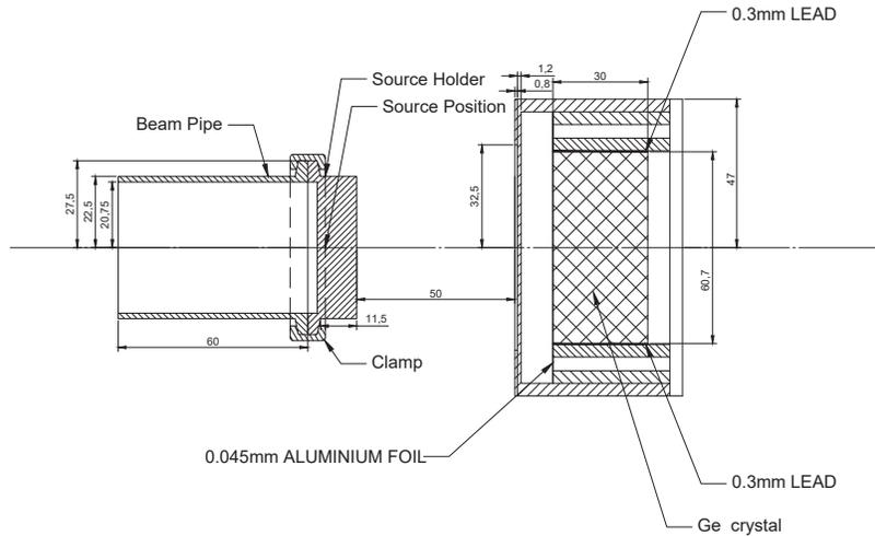
Figure 1: The internal structure for holding the Ge crystal: as provided by the manufacturer for the BEGe detector, source holder, and beam pipe geometry, are shown in this figure. These specifications are used in the simulation.
