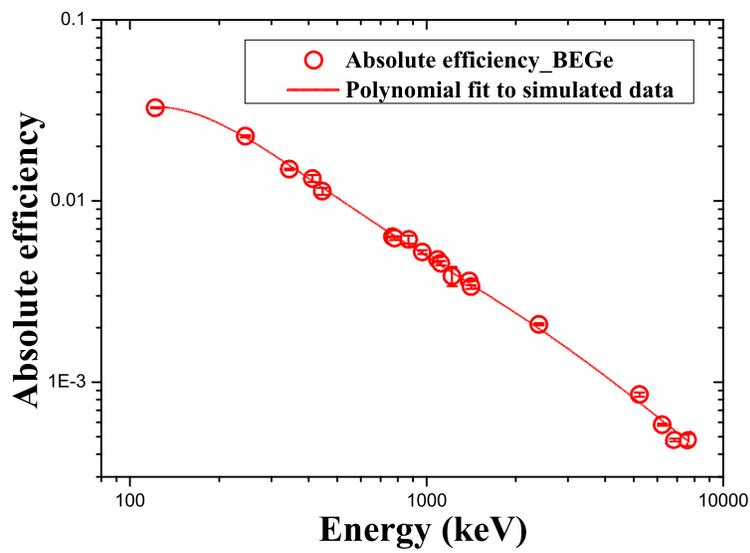
Figure 10: Simulated absolute detection efficiency values for  $^{152}\text{Eu}$  and resonance reaction  $\gamma$ -ray energies. Open red circles represent the results for Falcon BEGe detector. The corresponding error-bars are statistical errors calculated from the simulated photo-peak areas.
