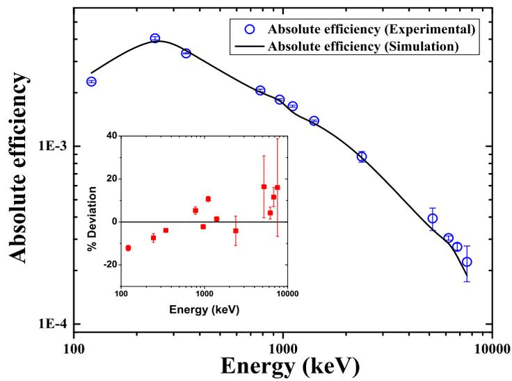
Figure 6: Absolute detection efficiency as a function of energy from 0.122 MeV to 7 MeV. Open blue circles represent the experimental data for Falcon BEGe at  $50^\circ$ . The corresponding error bars have been included in the symbols. The simulated results are shown with a solid line. The inset shows the percent deviation of the experimental data from simulated results. The errors in the deviation plot is only from the data.
