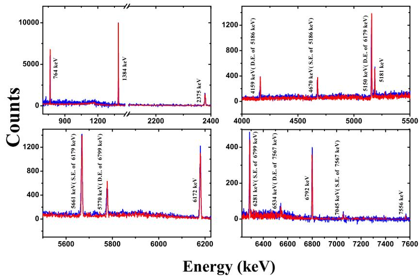
Figure 8: Comparison of experimental and simulated in-beam spectra at an angle  $50^\circ$  for the BEGe detector. The experimental and simulated spectra are drawn with red and blue curves, respectively.
