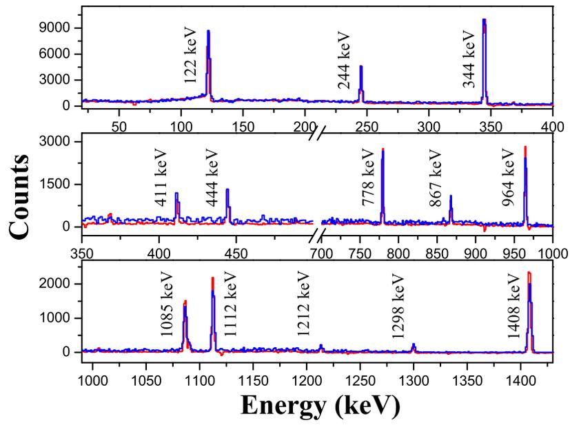
Figure 7: Comparison of experimental and simulated spectra at an angle  $50^\circ$  of  $^{152}\text{Eu}$  for the BEGe detector. The experimental and simulated spectra are drawn with red and blue curves, respectively.
